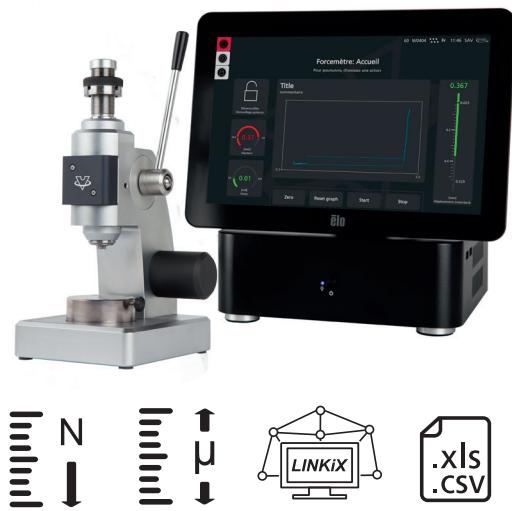
Characterization and control of driving in operations and spring elements through combined measurement of force and displacement. LINKiX®-compatible.
